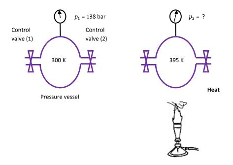
4. Gas in a 0.025  $m^3$  cylinder at 138 bar is reduced in volume to 0.016  $m^3$ . While heated from 297 K to 395 K, what is the final gauge pressure in the cylinder?
