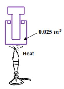
3. The constant volume vessel shown in Figure on which pressure gauge reads 138 bar is heated from 300 K to 395 K, what will the gauge read?
